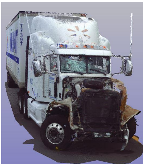
Figure 1. Three-dimensional scan of the Peterbilt combination vehicle involved in the June 7, 2014, crash in Cranbury, New Jersey.
